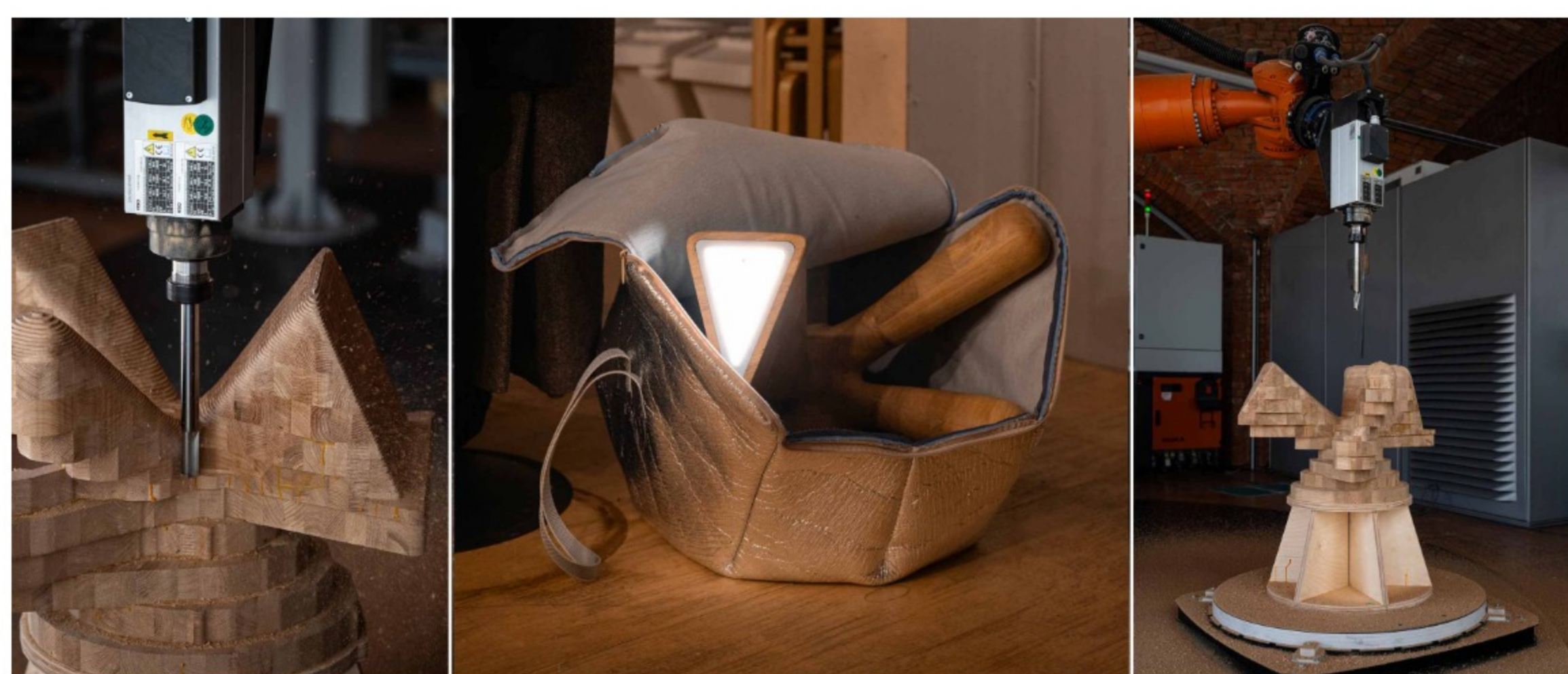
DICE is crafted and shaped by a robotic arm Image: Courtesy of KOSMOS Architects
